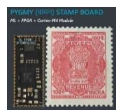
DORY Ad-hoc Mesh Radio ISM 865-867 MHz
